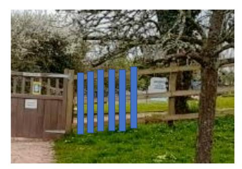
Slats to be attached to the existing fence rails, to keep dogs etc out, but allows wind to blow through. Approx. 1meter tall, inline with tops of posts.
